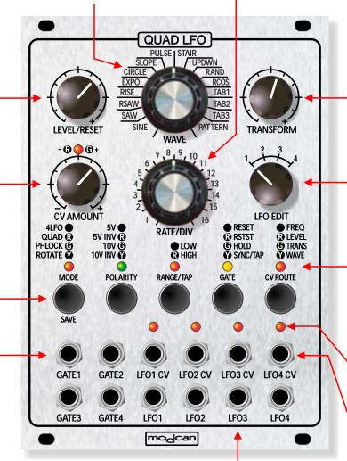
**LFO Outputs:** Output for each of the 4 LFOs. Output range can be changed with the Polarity switch from:
